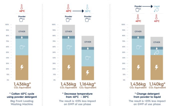
Global Warming lifecycle impacts vs key factors in use phase of a washing machine. Source: The Truth About Laundry, 2021
